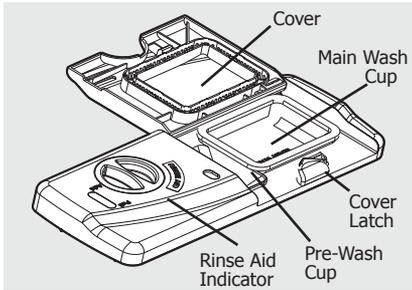
**If the cover is closed on the Main Wash Cup open by pressing the Cover Latch.**
