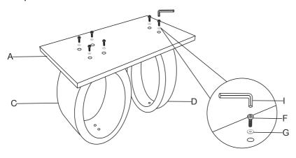
Firstly, fix the table leg with table base but do not fully tighten the bolt(F).
