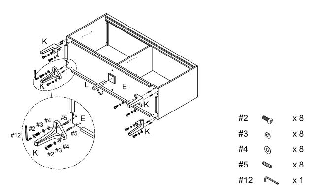
Step 6. Attach top panel (part A) to assembled unit (parts B, C2 & D) using wood dowels (part #5), short bolts (part #2), spring washers (part #3), flat washers (part #4) and allen wrench (part #12).
