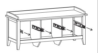
Slide out the side panel drawer glides for proper insertion of the drawers.
