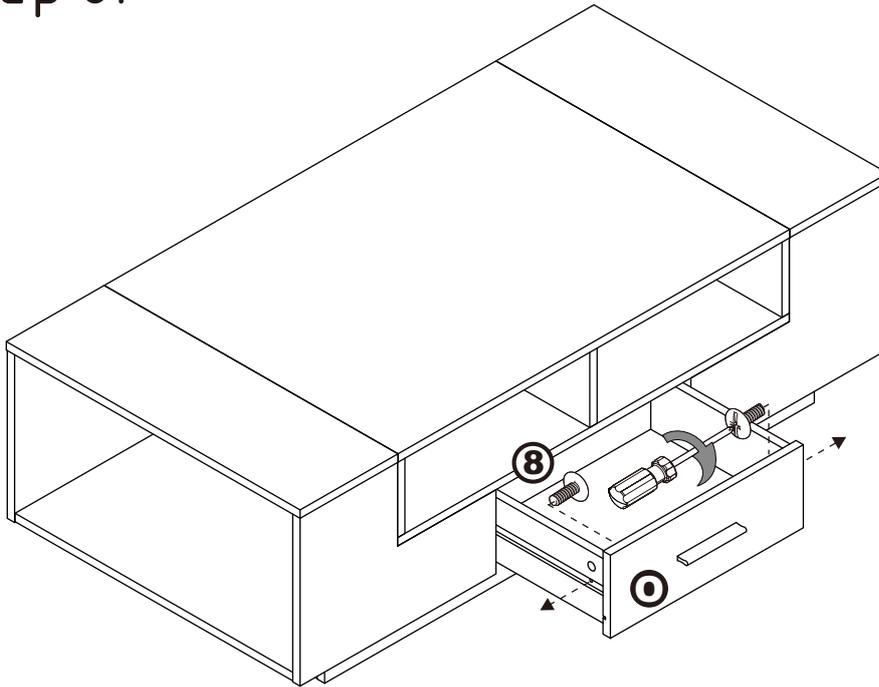
Extend the two outer slides of the runners so that they could align with the sides of the drawer. Make sure the pre-drilled holes from the drawer align with the screw holes of the outer slides. Secure two screws from the inside of the drawer using a Phillips screwdriver to tighten them to the outer slides.
