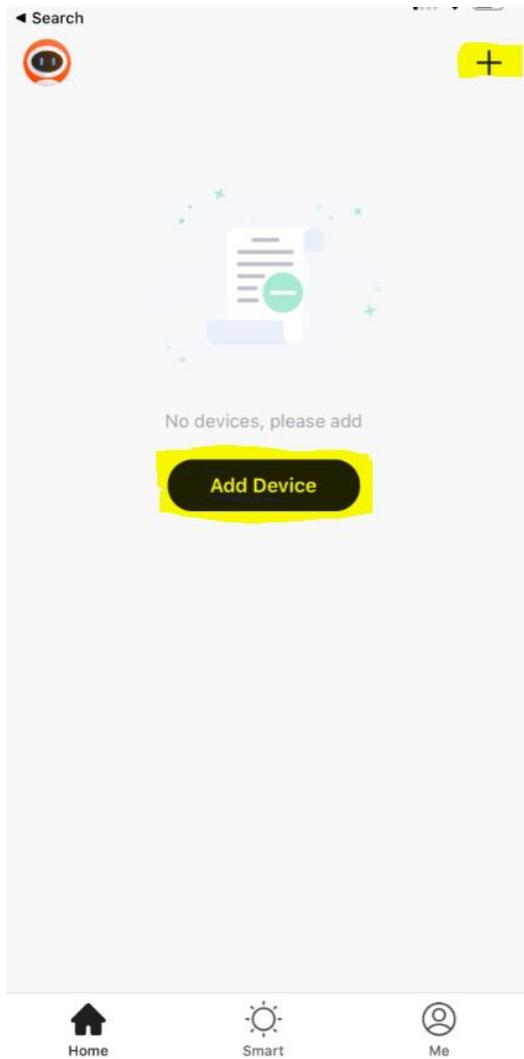
**3. You will be able to add device by pressing the '+' on the top right or on the main button in the middle.**
