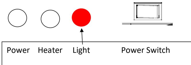
**6. Once back at the radar screen. Turn power on and press and hold, for a few seconds, the light control button on the top right-hand side of the unit.**
