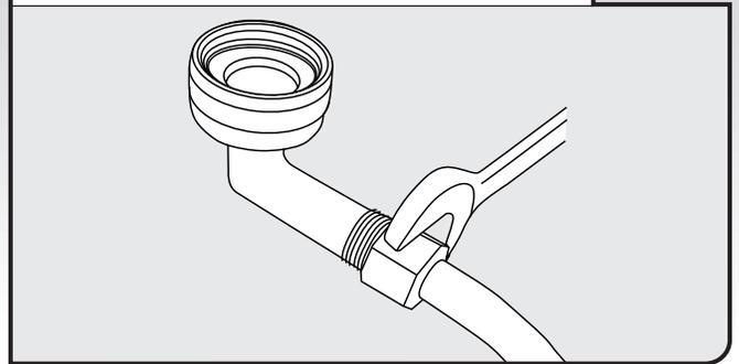
Connect the 3/8" compression fitting to the water supply line prior to installing the unit into the cabinet opening. Attach such that the 3/4" connection is facing upward as shown above.
