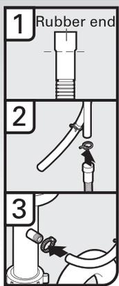
1. Connect rubber end of drain hose to air gap and cut if needed.
