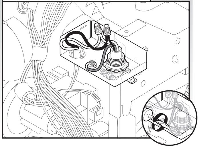
Tighten strain relief screws to secure cord.
