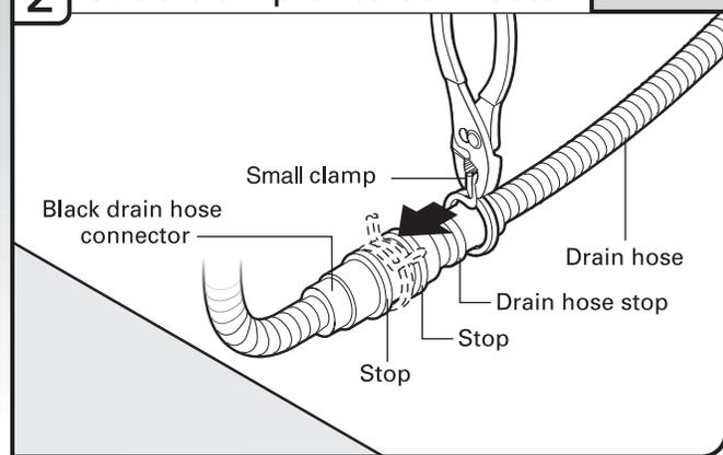
Using pliers, squeeze open the small drain hose clamp and slide onto connector between stops.
