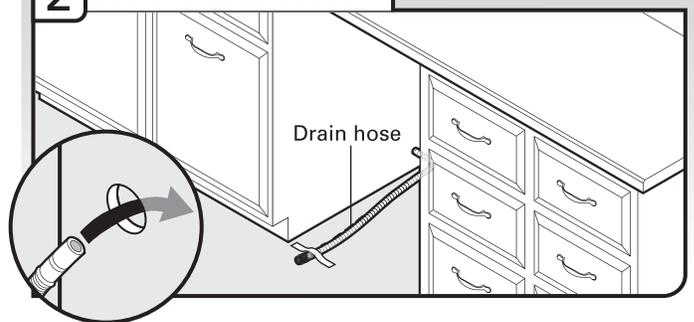
Route drain hose as shown through hole in cabinet to the front center of opening where drain connection will be made. Tape drain hose to the floor in area shown. This will prohibit it from moving when dishwasher is moved into cabinet opening.
