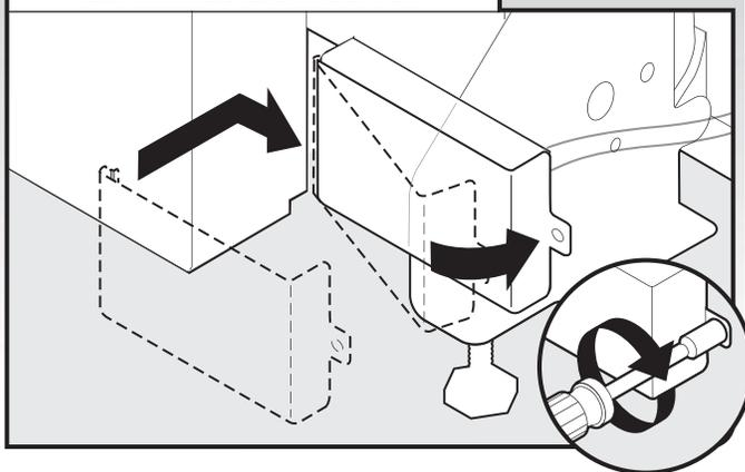
Place wires inside terminal box. Insert tabs on left side of cover. Make sure wires are tucked inside box. Close cover ensuring wires are not pinched. Use 1/4" nut driver or Torx® T20® screwdriver and previously removed screw to secure cover.
