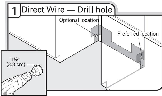
Drill a 1 1/2" (3.8 cm) hole in right-hand cabinet side or rear. See "Product and Cabinet Opening Dimensions" section.
