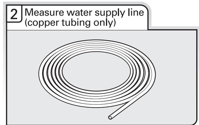
Measure overall length of copper tubing for the water supply line.
