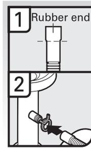
1. Fit rubber end of drain hose to waste tee and cut if needed.
