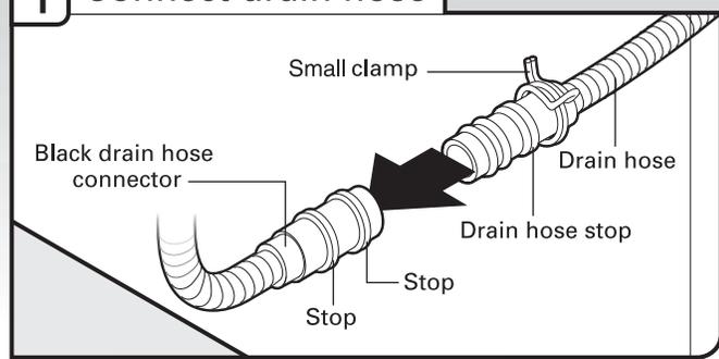
Place towel under drain hose to catch any water in drain hose. Place the small drain hose clamp onto the small end of the drain hose. Push the new drain hose into the black drain hose connector up to the drain hose stop.
