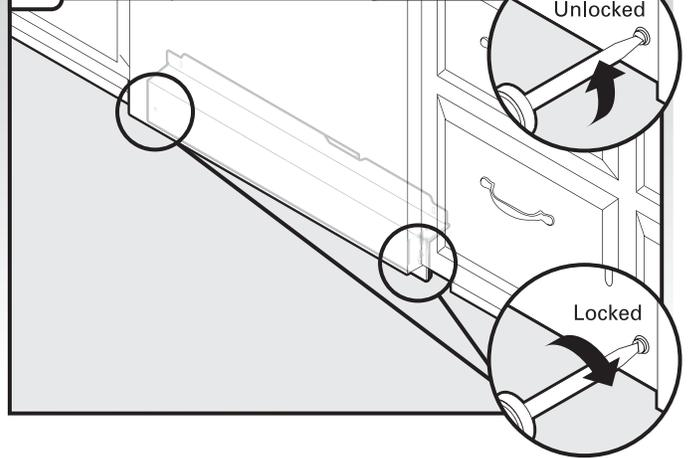
Using a flat-blade screwdriver, turn the fasteners  $\frac{1}{4}$  turn clockwise to lock into place. The fasteners slot will be straight up and down when properly locked.
