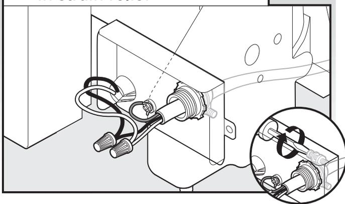
Tighten strain relief screws to secure cable.
