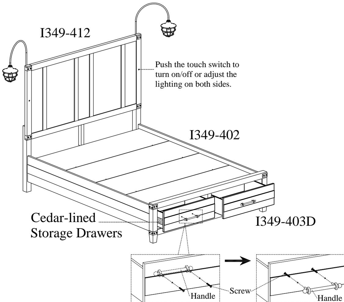
Reverse each handle by removing the screws while each drawer is open and attach all handles to the front of the drawers with screws as shown.
