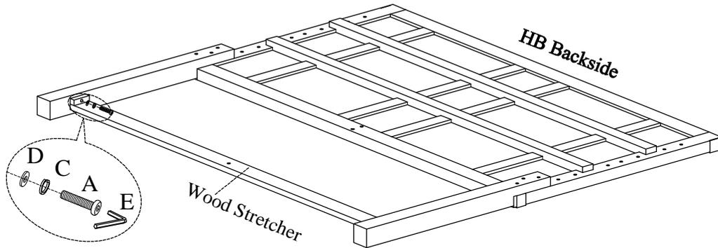
**STEP 3:** Attach the center support leg to headboard and wood stretcher by using 3 bolts(A), lock washers(C) and flat washers(D).
