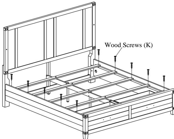
**STEP 9:** For the Cal King bed, both filler boards are notched. Using a utility knife only cut off the small piece at the notch on one of the filler boards. This cut off filler board will be placed at the foot of the bed going from left to right as shown on the right side below in STEP 10. For the standard King bed, skip this step and arrange the decking boards as shown below.
