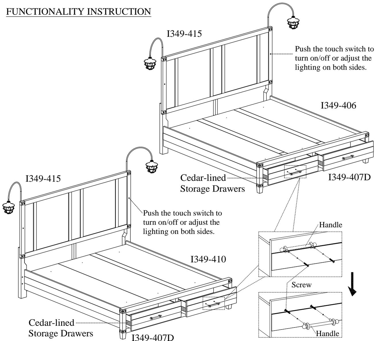
Reverse each handle by removing the screws while each drawer is open and attach all handles to the front of the drawers with screws as shown.
