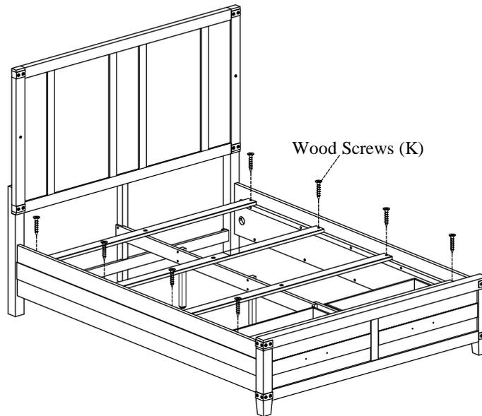
**STEP 9:** Put the decking over the slats, secure decking to the slats with wood screws (P) through the pre-drilled holes in the decking as shown below.
