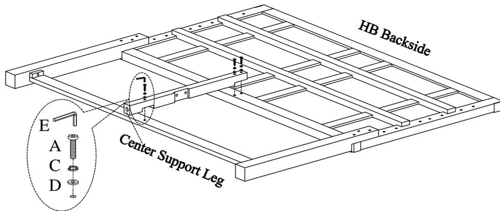
**STEP 4:** Put the footboard face down on a soft surface. Attach the support legs (for footboard) to the footboard as shown below.
