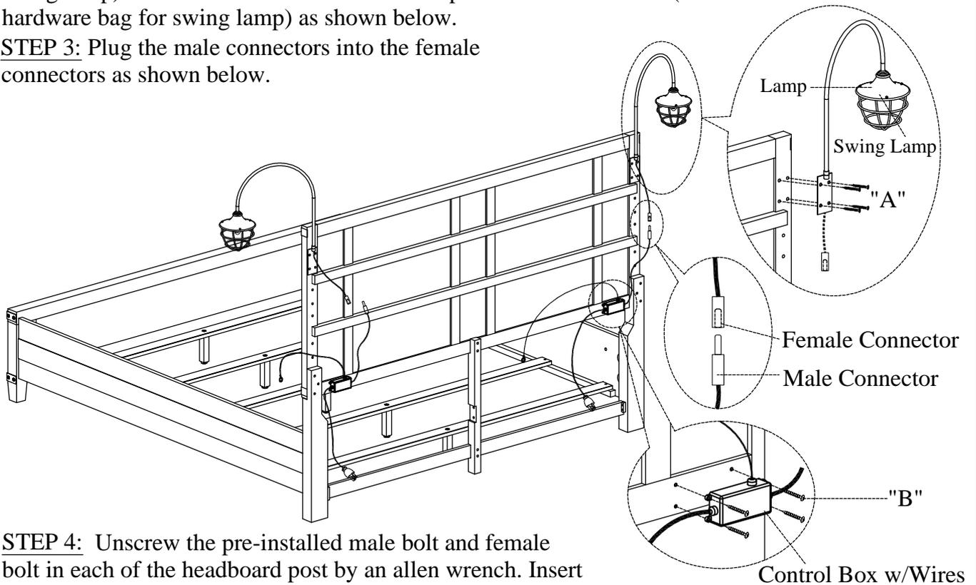
**STEP 4:** Unscrew the pre-installed male bolt and female bolt in each of the headboard post by an allen wrench. Insert each of the flat washer firstly and the brass ring secondly to the bolt male, press each bolt female/touch switch by finger into the hole on headboard post, then completely tighten the 2 male bolts.
