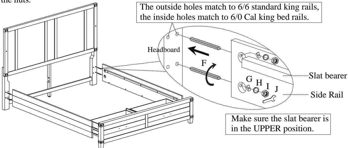
**STEP 6:** The standard king center rail(short) is in the Storage Footboard carton, and the Cal king center rail (long) is in the Cal King side rail carton. Attach the appropriate center rail to the footboard and center support leg of headboard using 4 bolts(M), lock washers(N) and flat washers(O).
