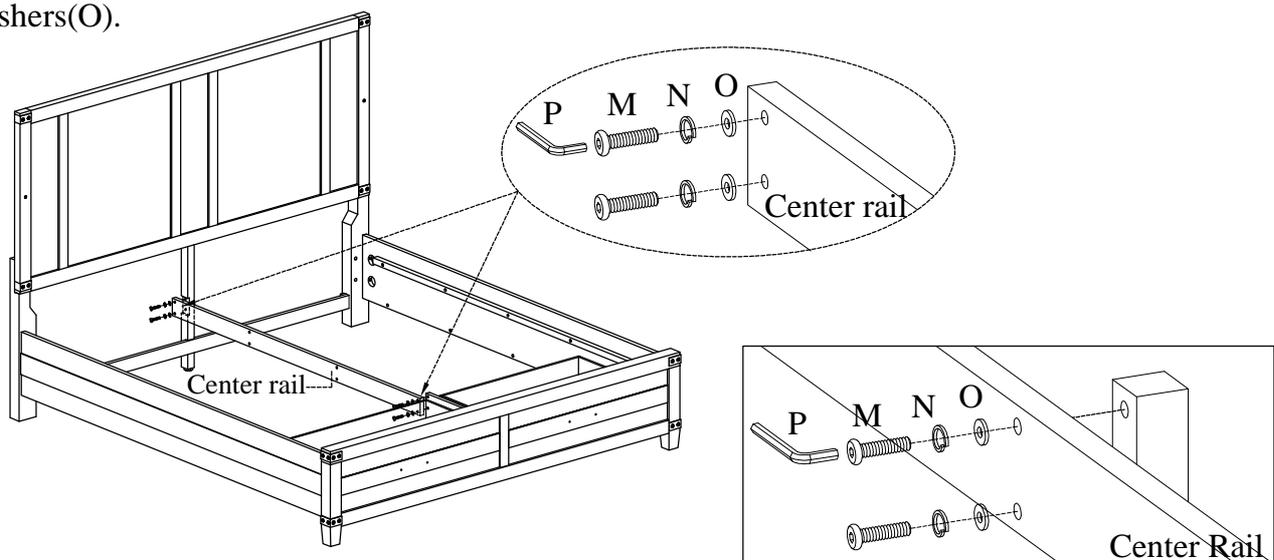
**STEP 7:** Attach 2 support legs (for center rail) to the center rail using 4 bolts(M), lock washers(N) and flat washers(O). Use the Allen Wrench(P) to tighten all of the bolts.
