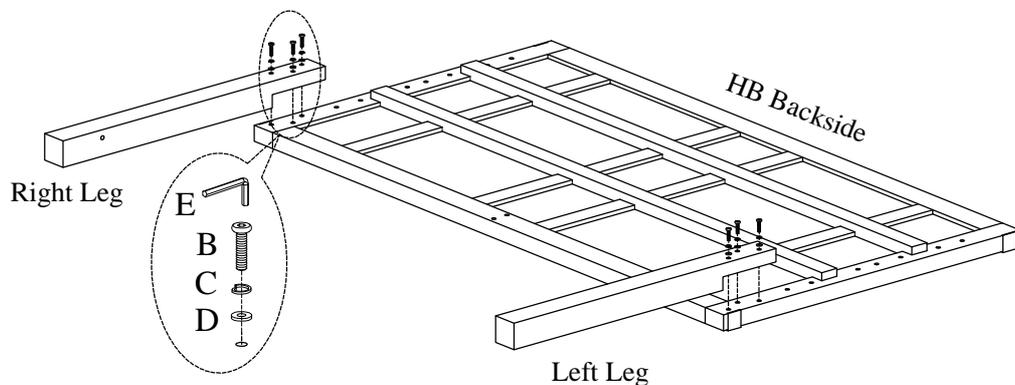
**STEP 2:** Attach the wood stretcher to the legs by using 2 bolts(A), lock washers(C) and flat washers(D). Completely tighten all bolts.
