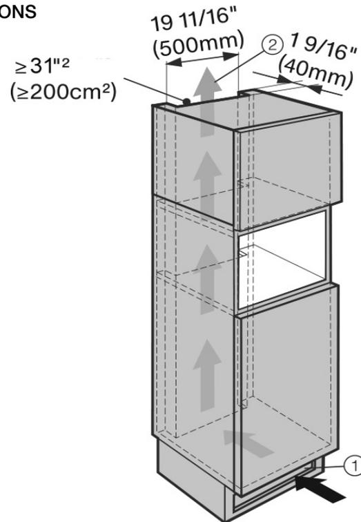
Air intake ① occurs via the plinth at the bottom of the appliance and the air escapes at the top ② at the rear of the surrounding cabinets.
