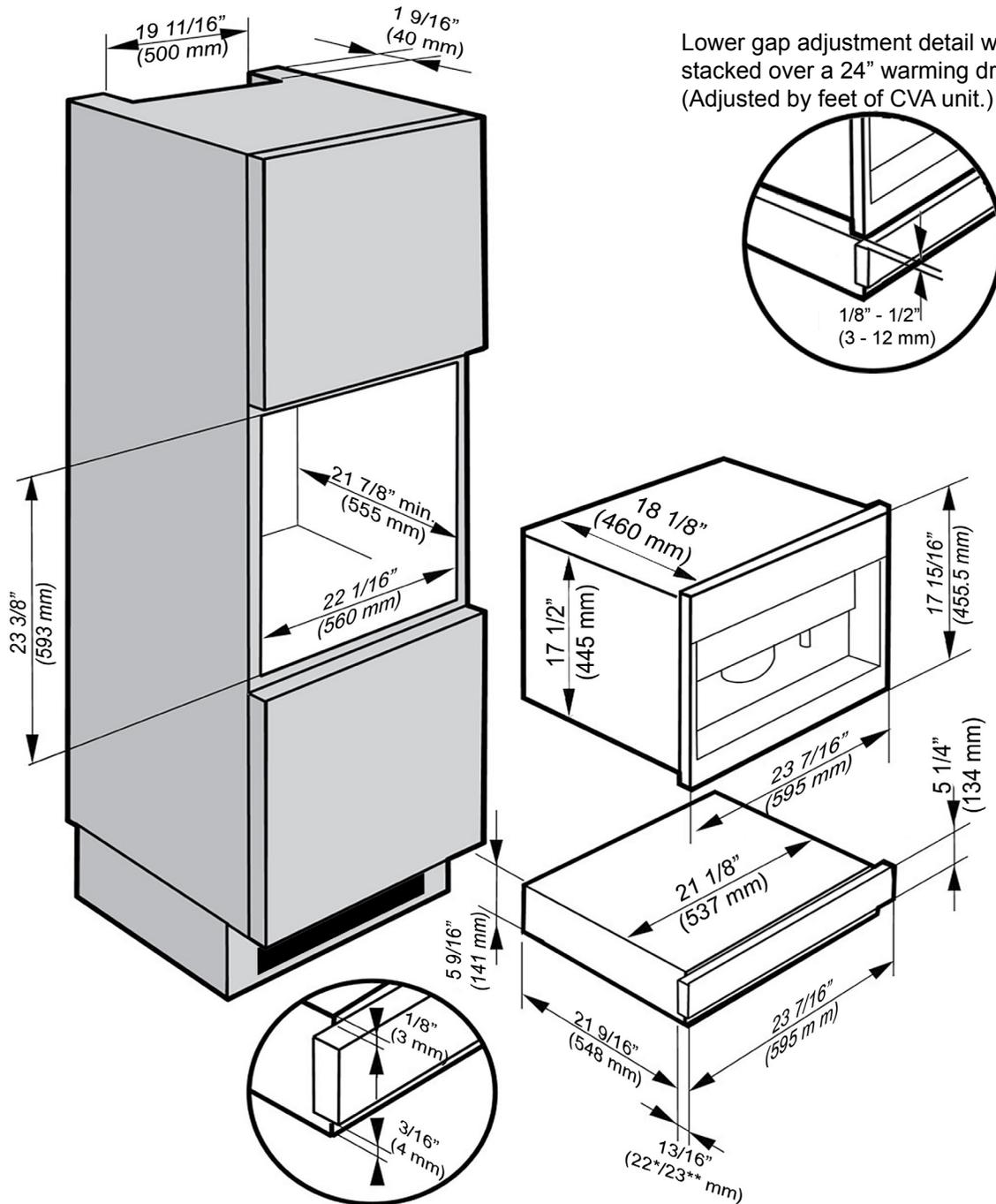
**PLEASE NOTE:** Condensation water can damage the coffee system or surrounding cabinets. The specified ventilation cross-sections absolutely must be observed.
