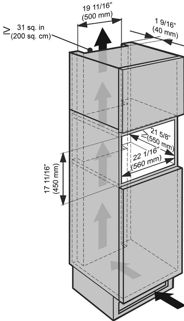
Lower gap adjustment detail when solo installed.
