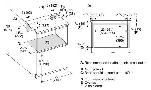
If under a counter, minimum clearance to counter top should be 7/16" (11 mm)
