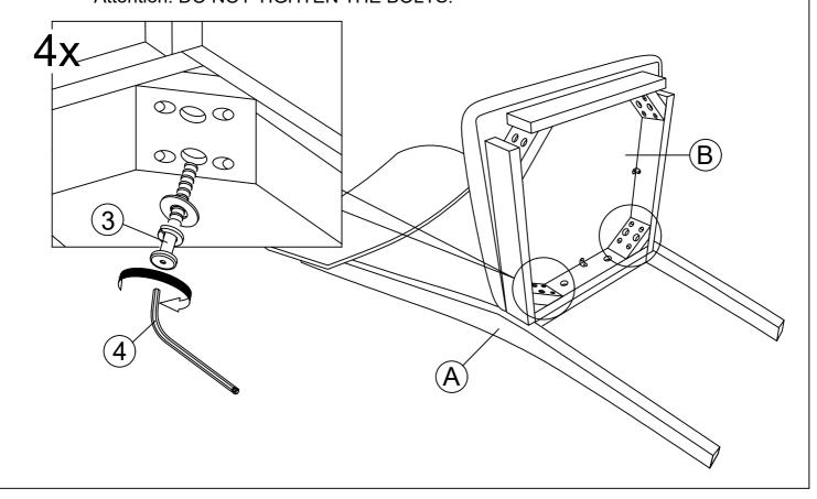
STEP 3 : Assemble the legs (C & D) with the seat frame with cushion (B) by using Allen key (4) with hardware (2).
