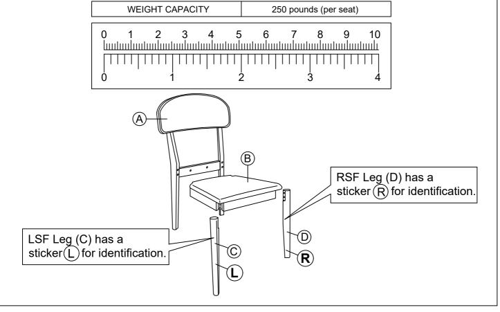
STEP 1 : Assemble the seat frame with cushion (B) with the chair back (A) using the Allen Key (4) with hardware (1).
