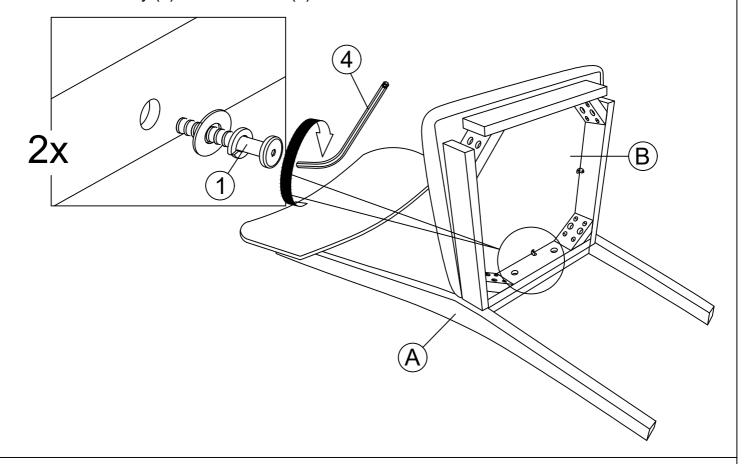
STEP 2 :Attach the seat frame with cushion (B) with the back legs of the chair back (A) by using the Allen Key (4) with hardware (3).
