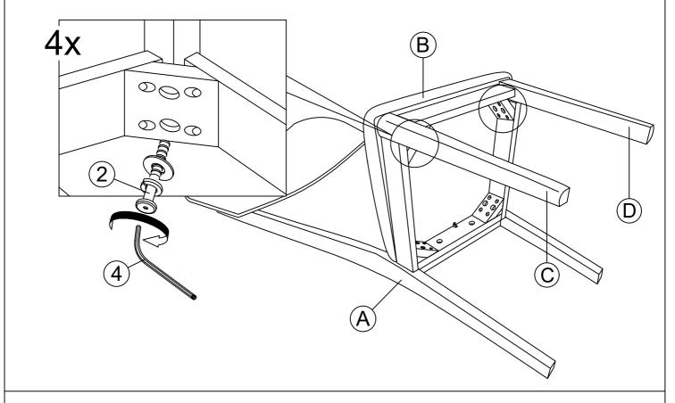
STEP 3: To level the chair, stand the chair up on a flat surface and tighten all the bolts by using Allen Key (4).
