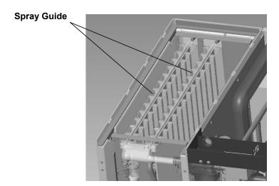
11) Refit the removed parts in the reverse order of the removal procedure. Check for water leaks.
