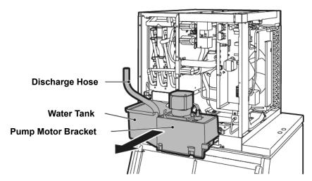
e. Remove the pump motor bracket securing the pump motor and the float switch. Remove the float switch from the pump motor bracket.
