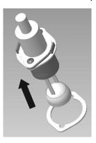
5) Attach the above float switch assembly to the pump motor bracket.
