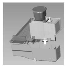
3) Flip over the pump motor bracket assembly, then twist off the float switch and pull out
