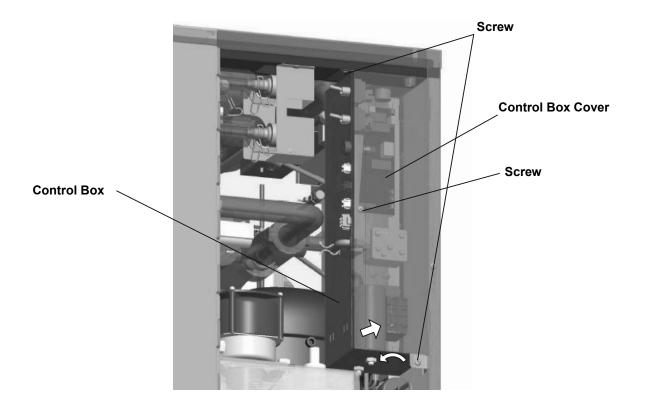
Note: After replacing the components inside the control box, connect and tie the wires properly in their correct position. Especially make sure that the harness does not press the push buttons on the control board.
