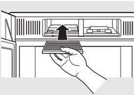
To install a new filter, remove plastic and other outer wrapping from the new filter.
