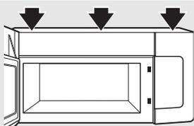
Remove 3 grille screws to remove the grille.
