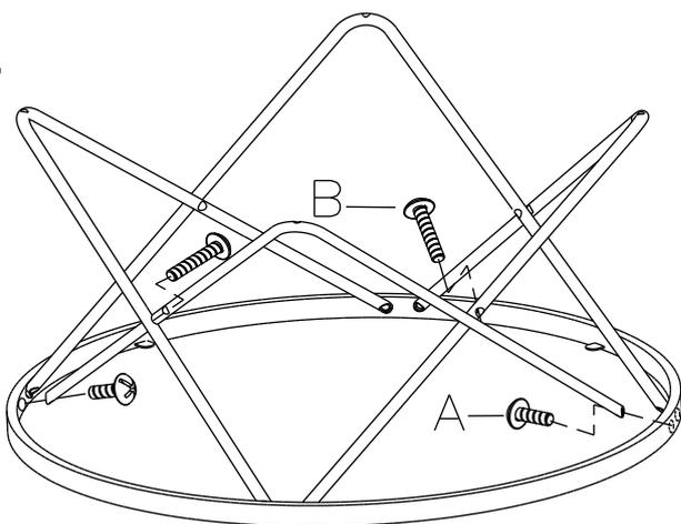
Repeat accordingly by using bolt (A) and bolt (B) again.
