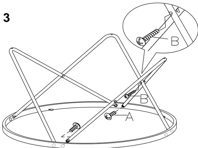
Repeat accordingly by using bolt (A) and bolt (B) again.
