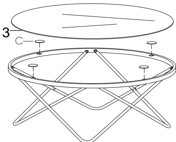
Turn the unit right side up and put glass pad (C) onto top frame as shown then put on glass top (3).
