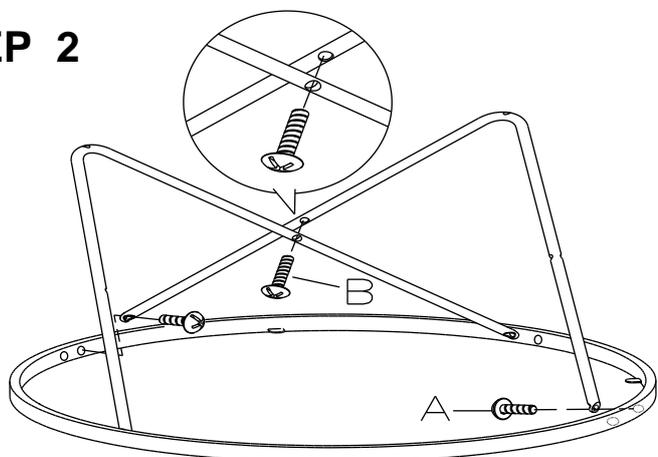
Repeat same step to attach leg (2) to top frame (1) by using bolt (A) and bolt (B) as shown.
