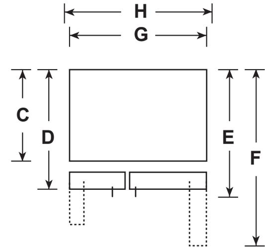
If installed against a wall, allow clearance of 14-3/16" on freezer side to remove bin.
