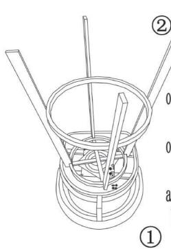
Step 1: Put the bolts(3) through holes of base and swivel.
