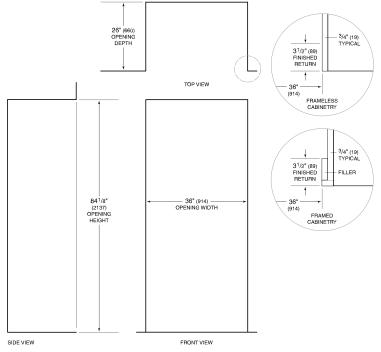
NOTE:  $3^{1}/2^{*}$  (39) finished returns will be visible and should be finished to match cabinetry.
