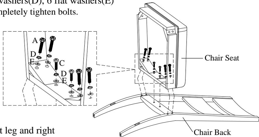
**STEP 2:** Attach the left front leg and right front leg to chair seat by using 4 bolts(B), lock washers(D), flat washers(E), Do not tighten bolts until STEP 3.
