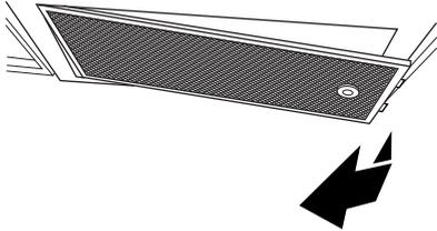
2. Replace grease filter by inserting one end of the filter into the left rim of the frame. Swing the right end of the filter up and slide it into position.
