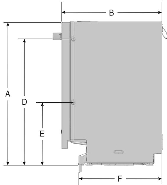
A. 32 <sup>1</sup>/<sub>4</sub> po-35 <sup>7</sup>/<sub>16</sub> po (820-900 mm) E. 14 <sup>1</sup>/<sub>16</sub> po (358 mm)
