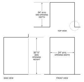
NOTE:  $3^{1}/2^{\circ}$  (89) finished returns will be visible and should be finished to match cabinetry.
