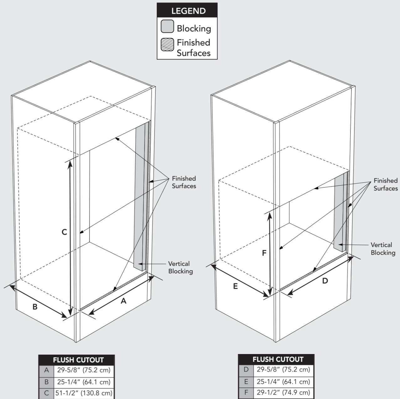
**\*Note:** To install the oven in a flush mount application the flush mount accessory kit (D30FTS for single ovens and D30FTD for double ovens) is required.
