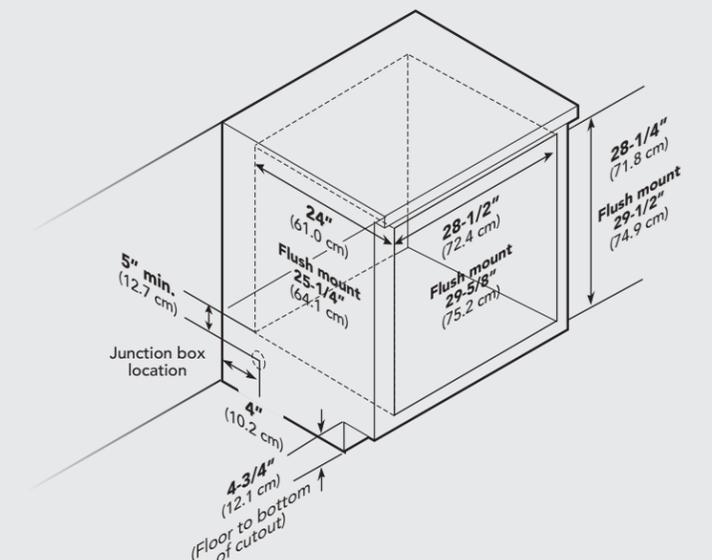
**\*Note:** To install the oven in a flush mount application the flush mount accessory kit (D30FTS for single ovens and D30FTD for double ovens) is required.
