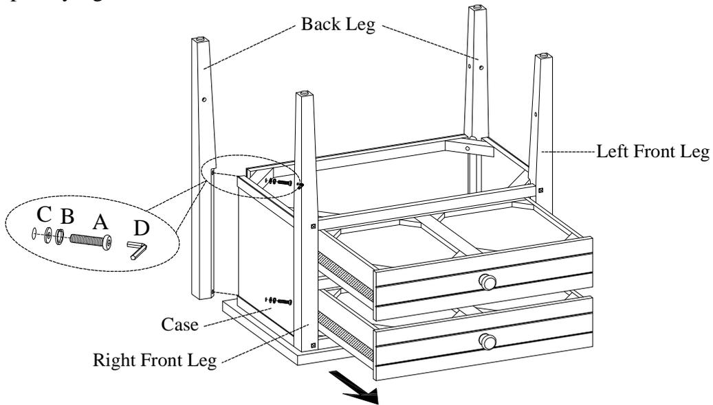
**STEP 2:** Attach the bottom frame and side stretchers to legs with 8 wood screws(E). Use the Allen wrench provided and the phillips screwdriver to tighten all the bolts and screws. Push back the drawers. Turn the assembled case to the upright position.
