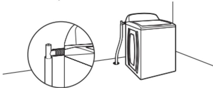
Floor drain system requires a Siphon Break Kit, 2 Connector Kits, and an Extension Drain Hose that may be purchased separately; refer to the Quick Start Guide for online ordering information. Minimum siphon break height: 28" (710 mm) from bottom of washer (additional hoses may be needed).
