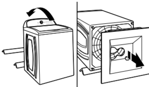
To avoid damaging floor, place cardboard supports from shipping carton on floor behind washer. Tip washer back and place on cardboard supports. Remove shipping base (some models require shipping base to be rotated 90° to the right before pulling off). Set washer upright.
