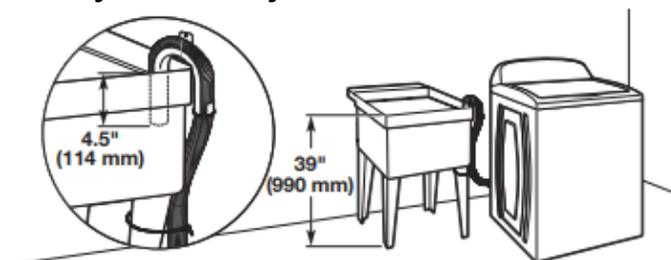
Minimum capacity: 20 gallon (76 L). Top of laundry tub must be at least 39" (990 mm) above floor; install no higher than 96" (2.44 m) from bottom of washer.
