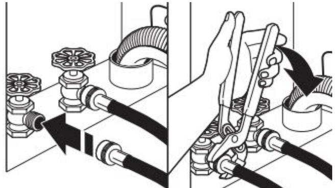
**IMPORTANT:** Do not overtighten hose or use tape or sealants on valve. Damage to the valves can result.
