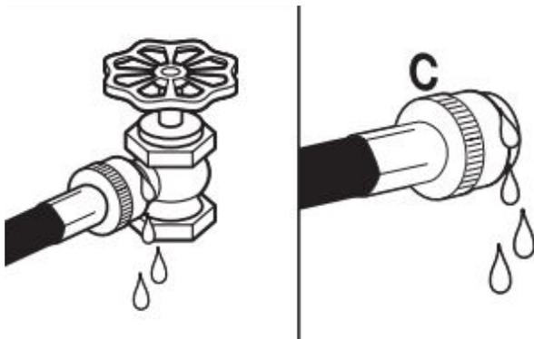
Turn on water faucets to check for leaks. A small amount of water may enter washer. It will drain later.
