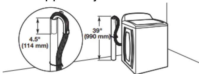
Minimum diameter for a standpipe drain: 2" (51 mm). Minimum carry-away capacity: 17 gallon (64 L) per minute. Top of standpipe must be at least 39" (990 mm) high; install no higher than 96" (2.44 m) from bottom of washer. If you must install higher than 96" (2.44 m), you will need a sump pump system.
