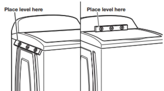
Move the washer to its final location. Place a level on top edges of washer. Use side seam as a guide to check levelness of sides. Check levelness of front using lid, as shown. Rock washer back and forth to make sure all four feet make solid contact with floor. If washer is level, skip to step 15.
