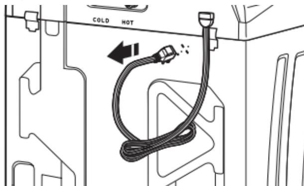
Firmly grasp power cord plug and pull to free from rear panel. Gently place power cord over console to allow free access to back of washer.
