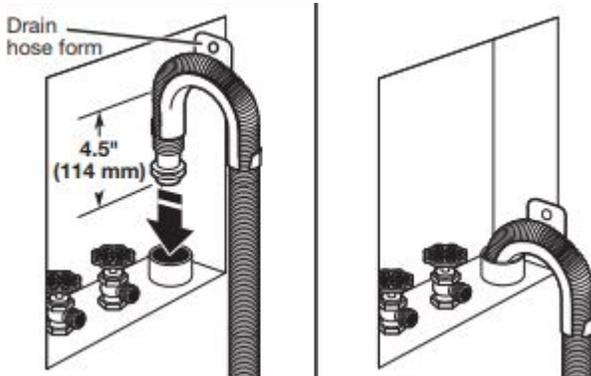
**IMPORTANT:** 4.5" (114 mm) of drain hose should be inside standpipe; do not force excess hose into standpipe or lay on bottom of laundry tub. Drain hose form must be used.
