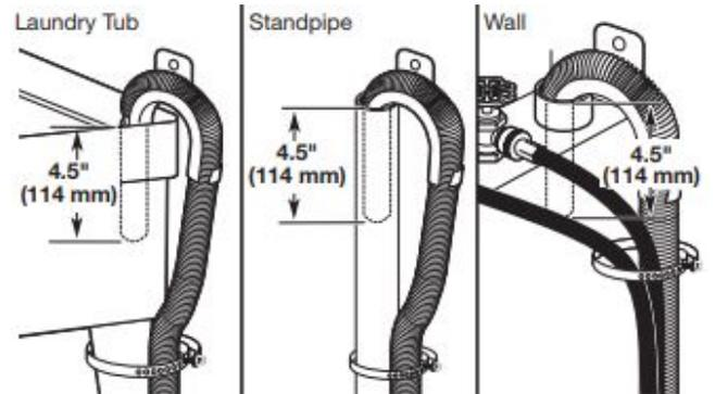
Secure drain hose to laundry tub leg, drain standpipe, or inlet hoses for wall standpipe with cable tie.
