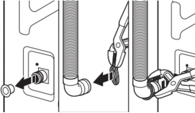
If applicable, remove the red plastic plug from the black drain port on the back of the washer.
