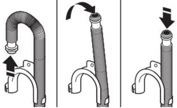
For floor drain installations, you will need to remove the drain hose form from the end of the drain hose. You may need additional parts with separate directions. See "Tools and Parts."
