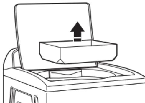
Remove tape from washer lid, open lid, and remove packaging material from washer tub. Be sure that all parts have been removed from inside washer.
