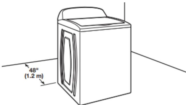
Move washer to within 4 feet (1.2 m) of its final location; it must be in a fully upright position.
