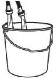
Run water for a few seconds through hoses into a laundry tub, drainpipe, or bucket to prevent clogs. Water should run until clear.
