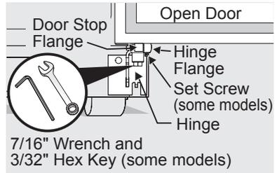
5. Reinstall the set screw, locking the door height.
