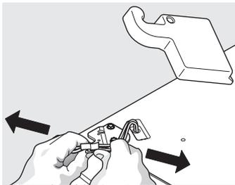
3. Trace lightly around the hinge with a pencil. This makes reinstallation easier.
