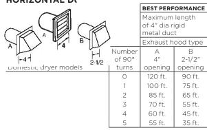
For every extra 90° elbow, reduce the allowable vent system length by 10 ft.
