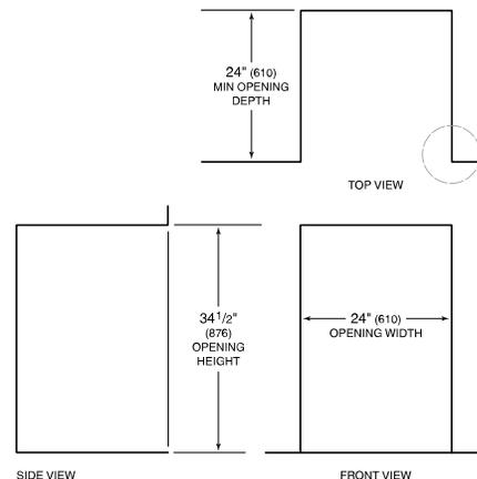
NOTE: 3/2" (89) finished returns will be visible and should be finished to match cabinetry.
