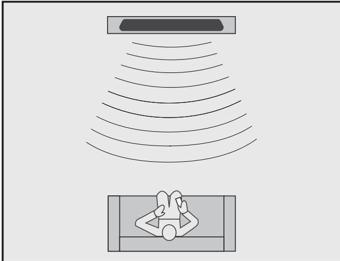
**Accurate Timbre:** For the most accurate and natural timbre, the speaker's high-frequency driver should be at, or aimed at, approximately ear level. Use the included optional leveling feet if you need to angle the SuperCenter so it points up (or down) at the listener.
