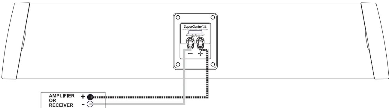
As shown above, hook up the center channel red(+) terminal of your receiver or amplifier to the red(+) terminal of your SuperCenter loudspeaker and the center channel black(-) terminal of your receiver or amplifier to the black(-) terminal of your SuperCenter. **It is essential that all speakers in your system be connected in the same way (in phase) to its own channel of the amplifier.**
