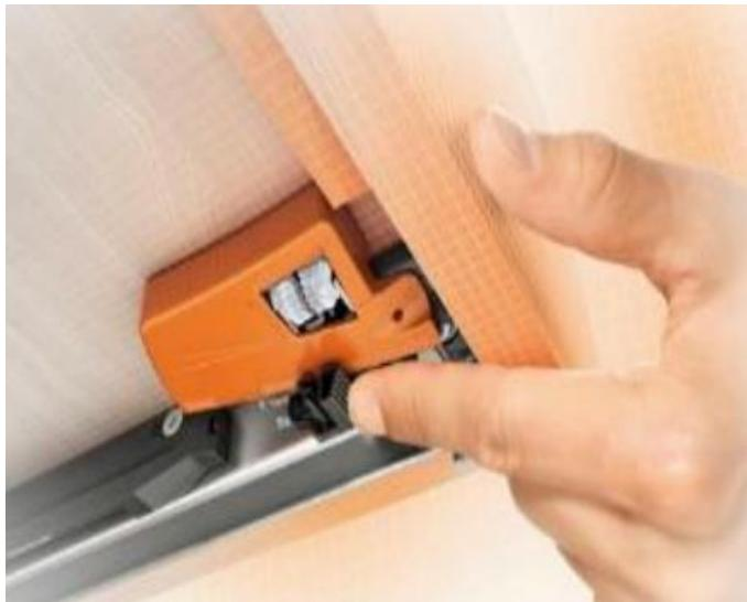
1) Adjust the gap from up and down that please push the plastic button then move front or back.
