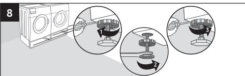
Using a level, make sure the units are level side to side and front to back. Do additional leveling as needed. Proper leveling keeps vibration at a minimum.
