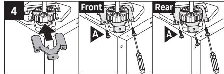
Attach a bracket Leg to each foot of the washer or dryer on the pedestal, and then secure it with two screws (A) at each front corner, and secure it with three screws (A) at each rear corner.
