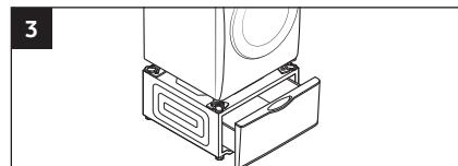
Turn the feet of the washer or dryer so that the feet are as close to the body of the washer or dryer as possible, then lock them in place. Place the washer or dryer onto the pedestal so that the feet rest properly in the clamps. See 3-a for the correct placement of the dryer and 3-b for the washer.
