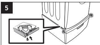
Attach a guide cover to each front corner of the pedestal and fasten it with screw (A).
