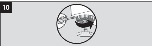
Once the washer is stabilized and does not vibrate, tighten the lock nuts on each leg of the pedestal using a flat head screwdriver.
