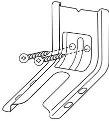
5. Using two #12 x 1 $\frac{5}{8}$ " Phillips-head screws provided, mount anti-tip bracket to the wall or floor.
