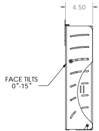
NOTE: CUSTOM INTERFACE BRACKET NOT SHOWN. THE CUSTOM INTERFACE BRACKET NEEDED FOR YOUR DISPLAY WILL ADD BETWEEN 1/2" AND 2" IN DEPTH AND MAY AFFECT LOCATION OF DISPLAY ON THE MOUNT.
