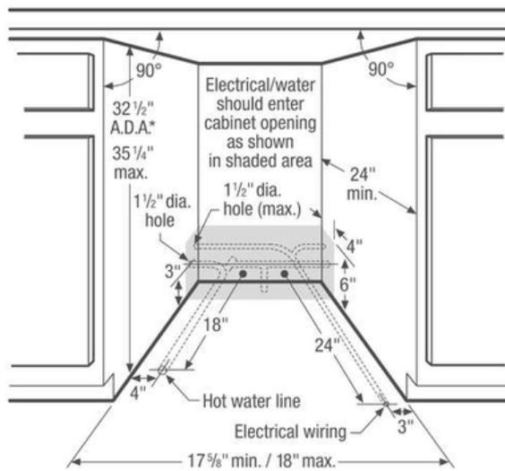
\*A.D.A. installation, (32 1/2") beneath 34"-high countertop may be accomplished by adjusting toekick and leveling legs.
