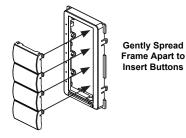
Attach button assembly to the device as shown in the following diagram. Ensure that LED strip is on the left side.
