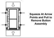
**NOTE:** When the button assembly is removed, power to the unit and load will be removed automatically.
