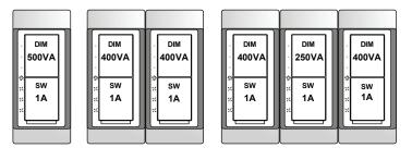
\* VA ratings are for input power to the transformer. If you do not know the input power requirement of the transformer, use the bulb's wattage rating to *determine proper rating*.
