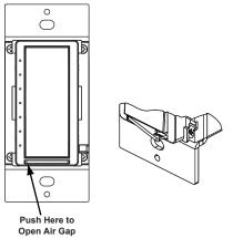
**NOTE:** Power is automatically disconnected when the button assembly is removed. For instructions on removing the button assembly, refer to "Changing Button Assemblies" on the previous page.
