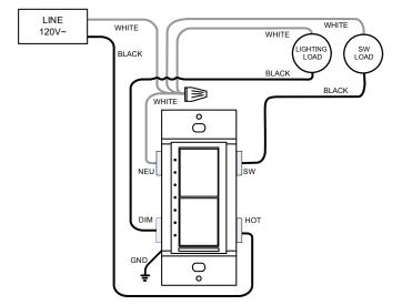
**NOTE:** Refer to the following diagram when making connections to the device.
