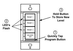
Operation described in this guide assumes the CLW-DIMSWEX-E is operating in "local" mode (without the use of a control system). The device can also operate in "remote" mode, where button behavior is dictated entirely by the control system program.
