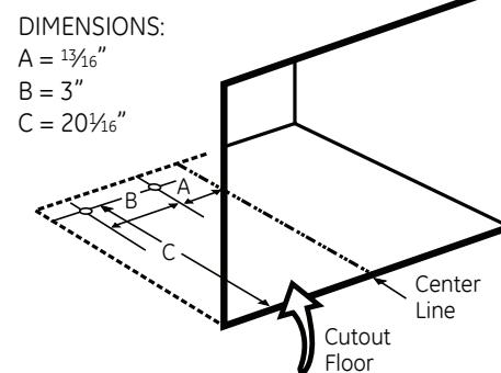
**C** Remove the template and drill two holes for the anti-tip brace.
