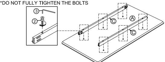
STEP 2: Install Table Leg (B) through pre-installed wood dowels at Long Apron (C). Then, assemble (C) to Table Leg (B) by using Allen Key (3) with the hardware (1).
