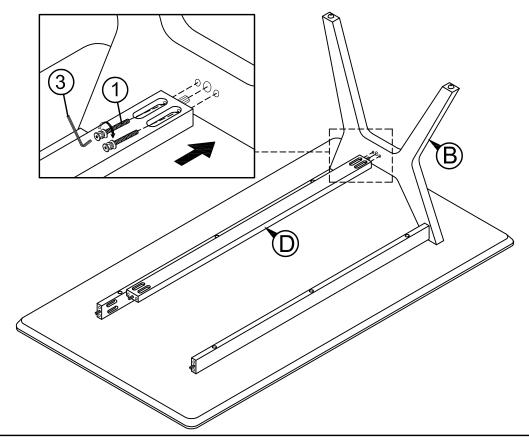
STEP 4: Install another Table Leg (B) Stretcher through pre-installed wood dowels at Long Apron (C) and Leg Stretcher (D). Then, assemble (D) to Table Leg (B) by using Allen Key (3) with hardware (1).
