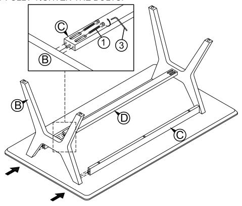
STEP 5: Assemble Long Apron (C) to Table Leg (B) by using Allen Key (3) with the hardware (1). \*PLEASE FULLY TIGHTEN THE BOLT NOW.
