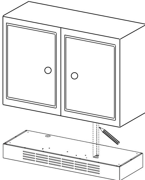
**2** Drill a hole for the electrical cable (bigger than the power cord strain relief).
