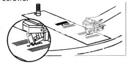
**VTA Adjustment:** To adjust the VTA, lay a record on the platter (15). Slacken the horizontal adjustment screws (two **Allen** screws located in the 11 and 1 o'clock position in the tonearm (10) base with the Allen Key provided.
