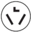
3-wire receptacle (10-30R)
