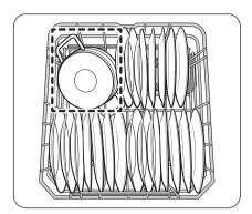
For more effective cleaning, load larger items into the Storm Wash<sup>+</sup> area on the left side of the lower rack (Dotted zone).
