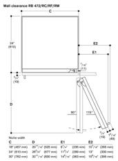
The drawing is based on a cabinet panel width of  $^3/4^\circ$  (19 mm) and a Gaggenau cabinet handle height of  $1^5/16^\circ$  (49 mm).
