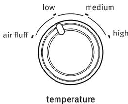
Select temperature by turning the knob to the desired position or select the Automatic Dry Cycle that has the temperature included in the cycle selections. See "Setting the Drying Temperature".
