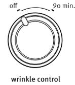
Select Wrinkle Control by turning the knob to the desired position.
