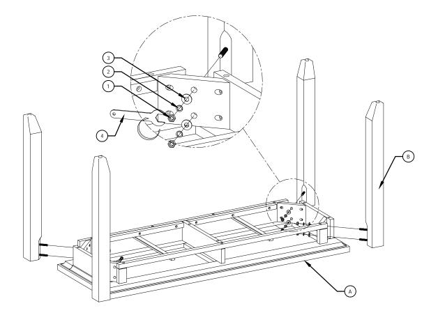
Step 2: Attach leg(B) into the top table(A). insert the hexagonal nut(1), lock washer (2), flat washer (3) into bolt, tighten with wrench(4).
