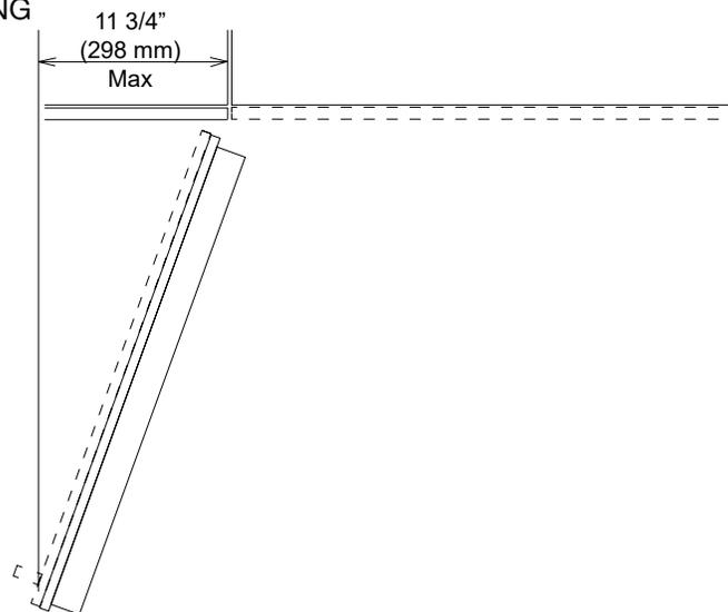
**NOTE:** Additional space needed depending on thickness of front panels and handle used
