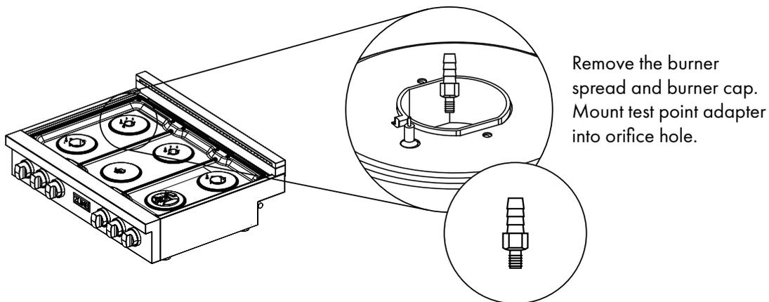
**NOTE:** If the test point adapter or 1/4" (6 mm) tubing was not included with your range top's Liquid Propane Gas Orifice Kit, please contact ZLINE Customer Experience at 1-614-777-5004.
