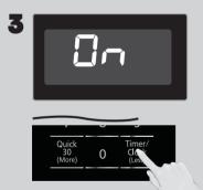
Press **Start** once, then Press **Timer/Clock (Less)** to cycle between the Beep on or Beep off.
