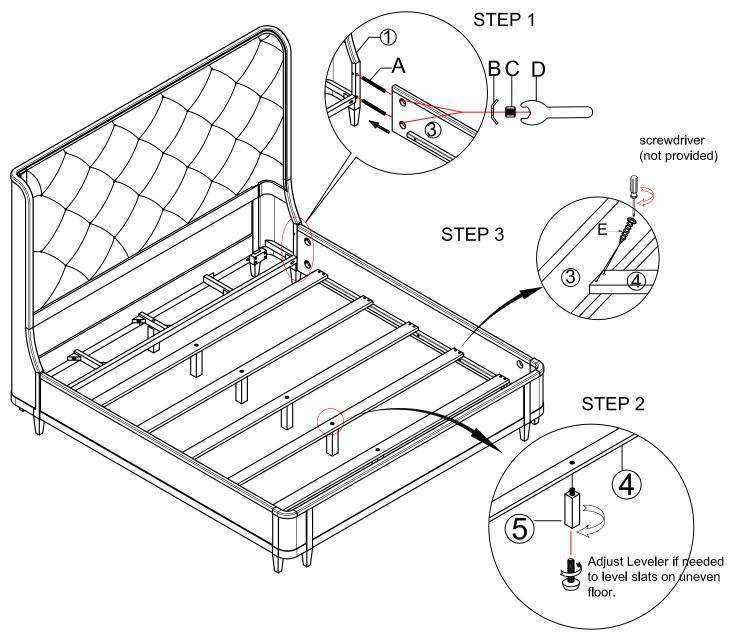
Step 1: Attach Rails (3) to Headboard (1) and Footboard (2) by using Threaded Rods (A), Curved Washers (B) and Nuts (C), tighten them with Open Wrench (D).
