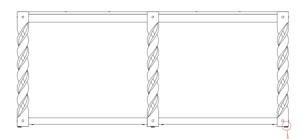
Adjust leveler if needed to level table on uneven floor.
