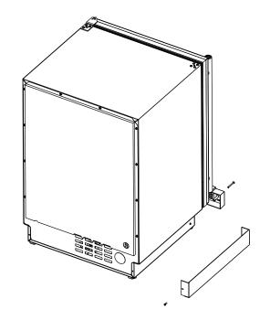
3. Align front hole with hole in shell accessory, hole in base, and hole in grille. Tighten screw.
