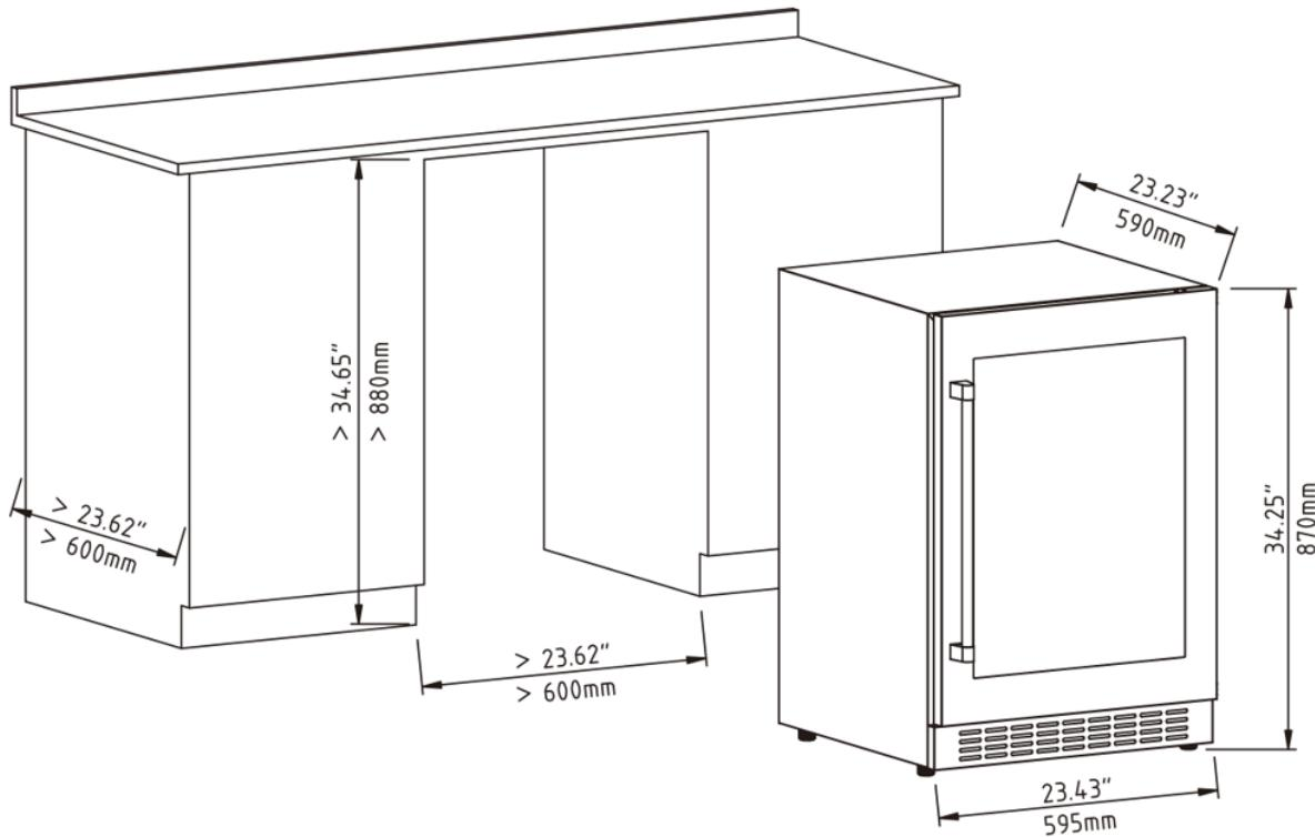
Note: If the appliance is fully built in and installed with a kitchen plinth, ensure that the ventilation openings in the plinth provide at least 300 cm<sup>2</sup> of free airflow. Remove any ventilation grilles so that hot air can disperse without obstruction. Otherwise, the appliance will operate under higher strain, leading to increased energy consumption.
